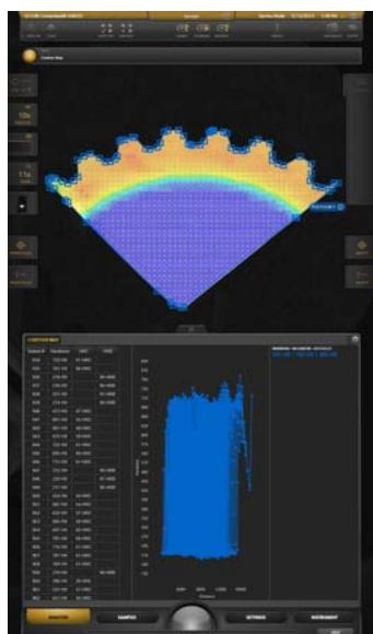
*Optional Color Hardness Contour Map displays sample hardness and location with a color representation of hardness variances.*
