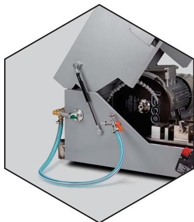
Supports 9 in (230 mm) and 10 in (250 mm) blades with 1.25 in (32 mm) arbor hole @ 3 hp (2.2 kW) with integrated electronic mechanical braking system
